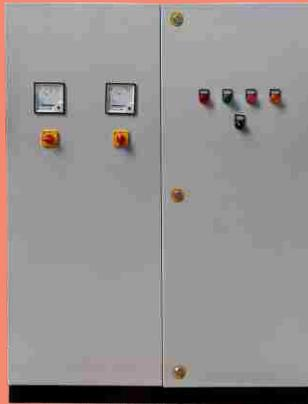
Starter is similar to Start- Delta Starter but a set of Series Reactors are connected in series with the motor winding while starting. So this method is often called as Series Reactor Starter. Once the motor comes to its running mode these reactors are disconnected and the motor runs like DOL method. The starting current is controlled by the Impedance produced by reactors connected in series.
