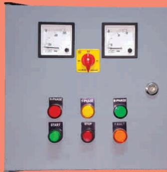
Start-Delta starters are the most common starters used widely to start AC motors. In these starters the starting current is controlled by applying reduced voltage, achieved by connecting motor winding in "Star" mode. Theoretically the current is reduced by a factor of  $1/\sqrt{3}$  times and once the motor attains its normal running stage, full voltage is applied to the motor by changing the connection to "Delta" mode and remains in the same stage till the motor is stopped.
